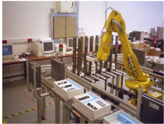
Figure 2: Factory Automation Laboratory showing part of the Packing Cell.
